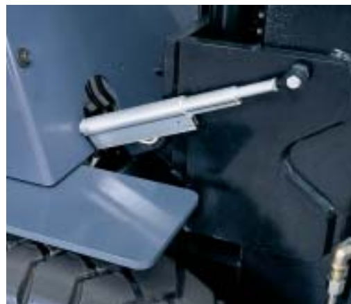
Tilt indicator mounted between cowl and mast.
