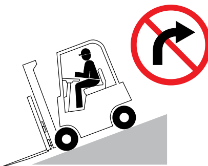
No turning on ramp
