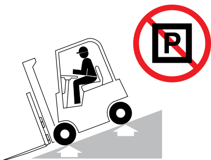
No parking on ramp
