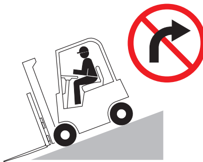
No turning on ramp
