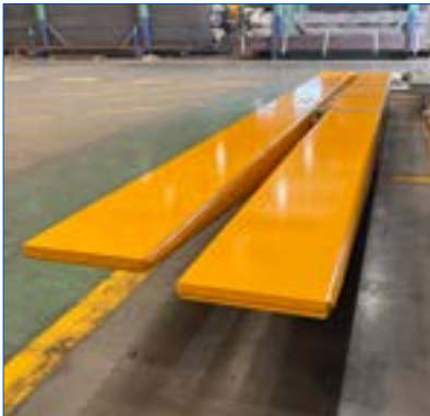
12mm welded steel plate
