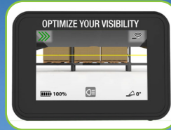
Adjustable horizontal target line and fork tilt angle indicator
