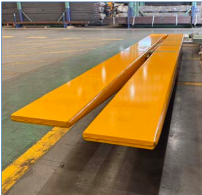
12mm welded steel plate
